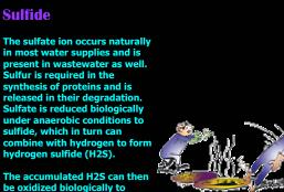
The accumulated H2S can then be oxidized biologically to sulfuric acid, which is corrosive to sewer pipes.
